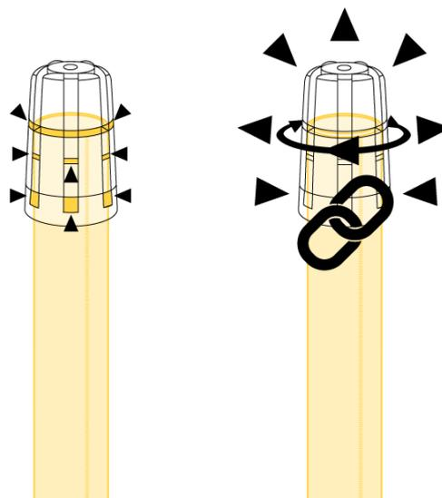
The tip is mechanically attached to the ejector trough the perfect interlocking of hooks integrated into the tip mould. The ejector does not allow the tip to come off, blocking its position persistently.
