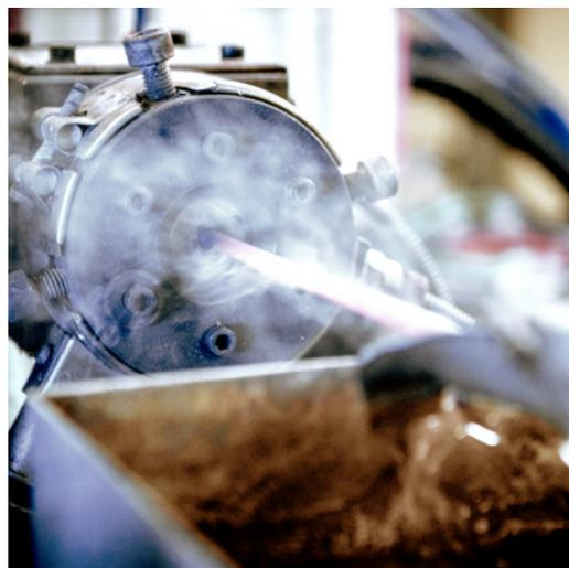
The inner wire is fastened to the tube without glue, as other manufacturers do. It is fused into the plastic during the production process.
